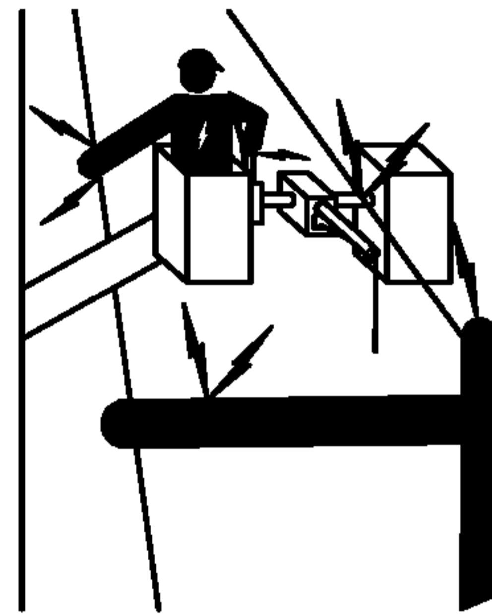
A pictogram illustrating a potential electrical hazard. It shows a worker standing on a lift platform, which is labeled as a 'double working platform with material handling system'. The worker is positioned near several parallel lines, representing power transmission lines. A lightning bolt symbol is shown above the worker, indicating the risk of electric shock or arcing. |
