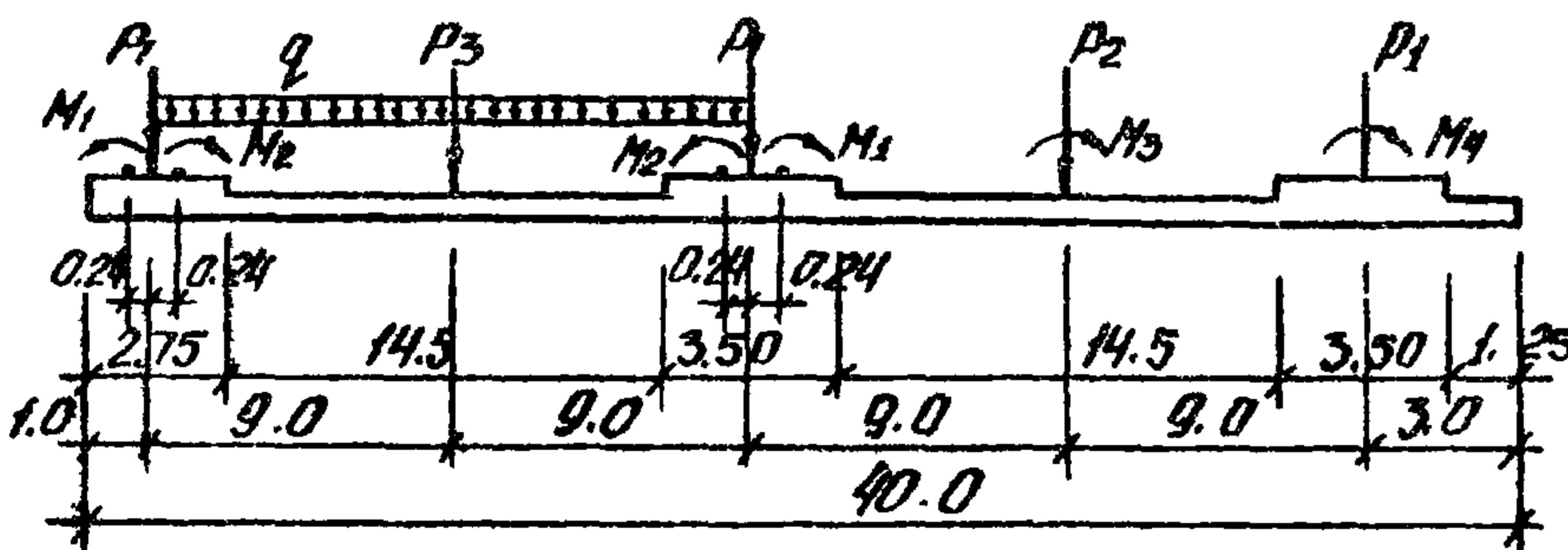
$$P_1 = 2.67 \text{ т} \quad P_2 = 5.45 \text{ т} \quad P_3 = 3.52 \text{ т} \quad q = 5.11 \text{ т/п.м.}$$
