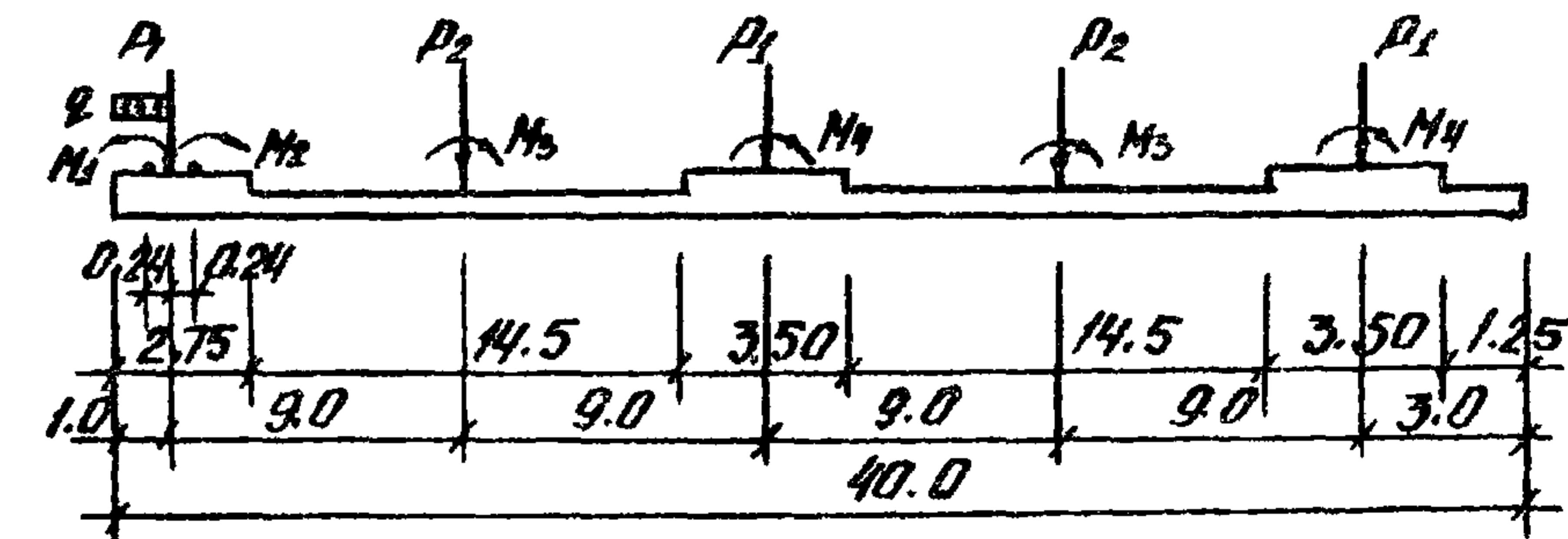
$$P_1 = 2.67 \text{ т} \quad P_2 = 5.45 \text{ т} \quad q = 11.0 \text{ т/п.м.}$$
