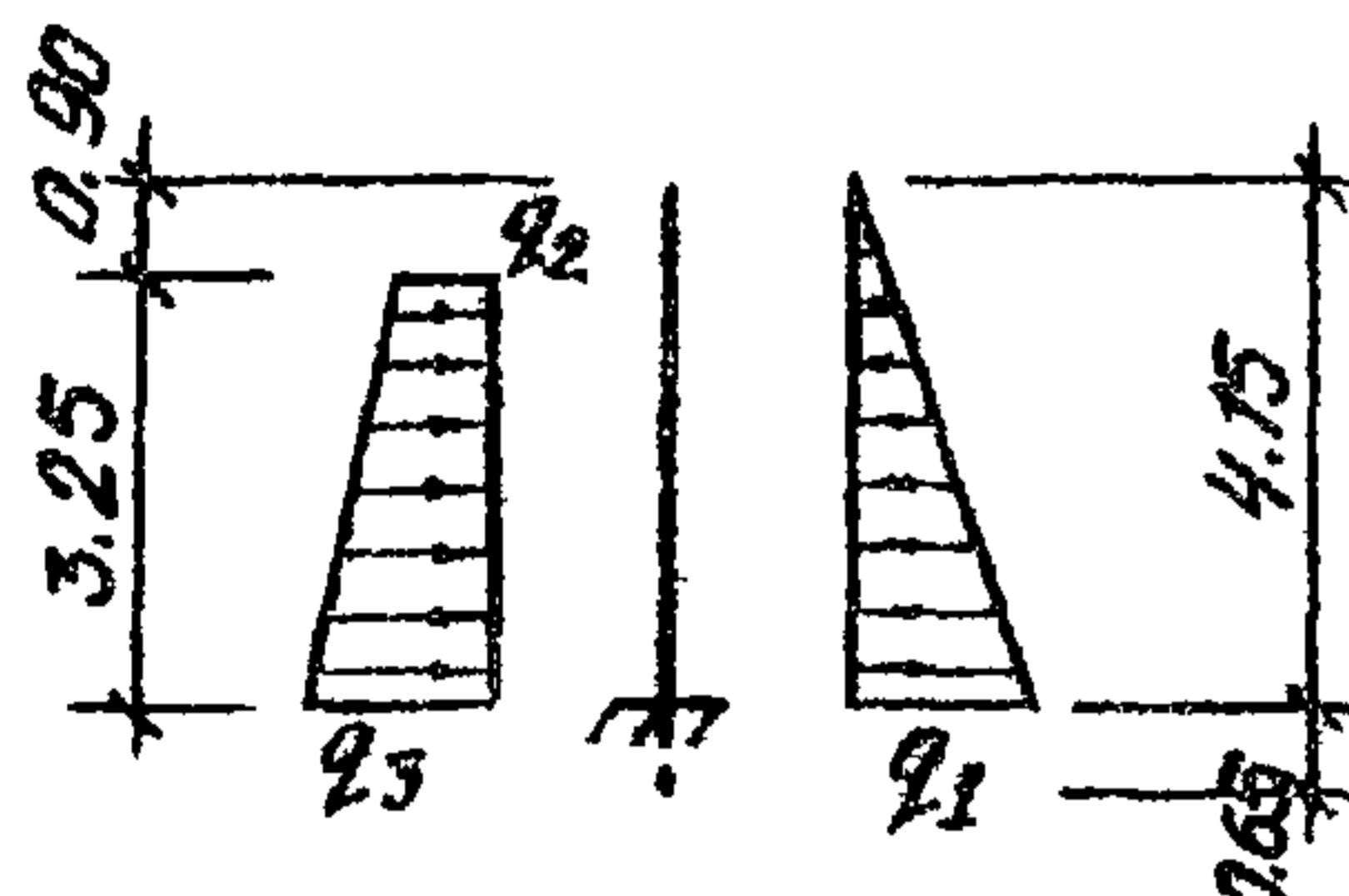
$$q_1 = 4.15 \text{ т/п.м.} \quad q_2 = 0.64 \text{ т/п.м.}$$
