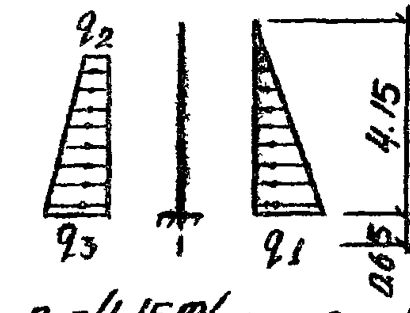
$$q_1 = 4.15 \text{ т/п.м.} \quad q_2 = 0.64 \text{ т/п.м.}$$
