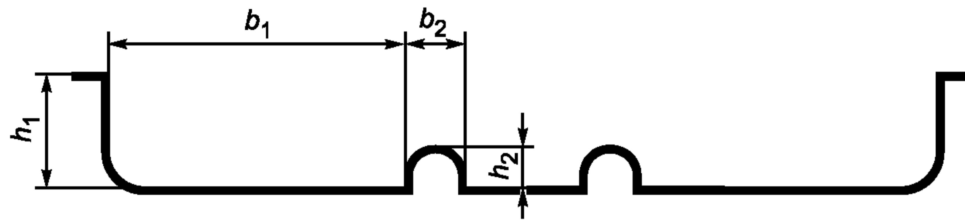
$$600 \leq b_1 \leq 1800; \quad h_1 \geq 500; \\ b_2 \geq 200; \quad h_2 \geq 200$$
